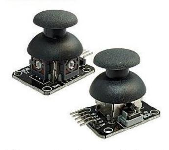
PS2 game rocker rocker arm module Electronic building blocks standard interface and 2.54 mm pin interface leads.
